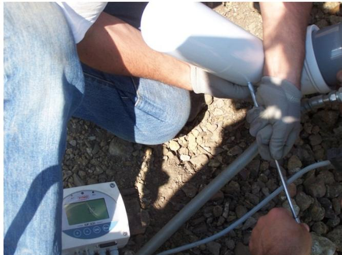
Figure 3 - Measurement of the dynamic pressure of the air entering a burner (with a Pitot tube)
