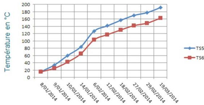
To increase the efficiency of the treatment, an insulation layer has been placed on the entire installation. Thus, to monitor ground-level temperatures, a thermocouple was placed between the concrete and the insulation layer.
